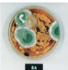
Microbiological swabs of insufficiently dewatered diesel samples
